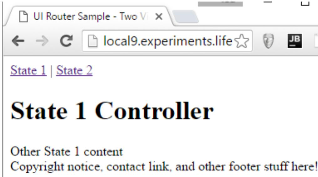
The app loaded into the default state of State 1. You can see the navigation bar up top and the footer at the bottom, with the main content in the center. Click the State 2 link:
